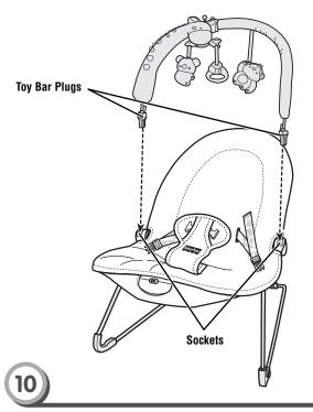
• Insert and "snap" the toy bar plugs into each retainer socket. Hint: The toy bar is removable. Press the ends of the latches and lift the toy bar.
